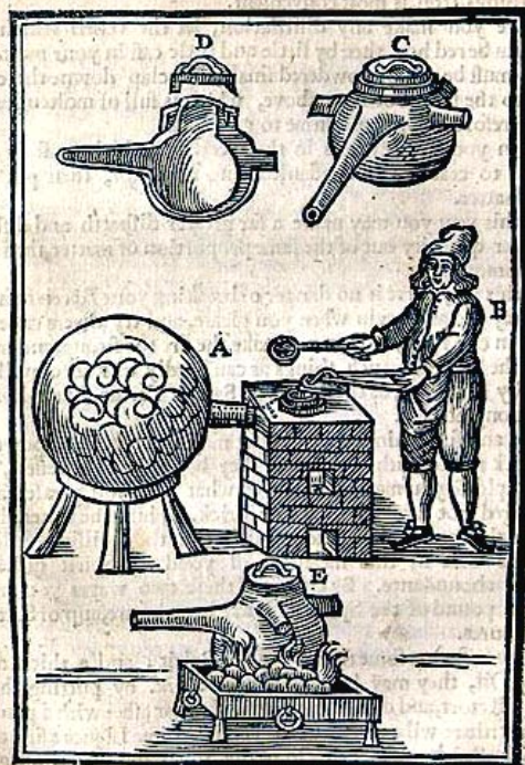
A, Signifies the Furnace with iron, or earthen distilling vessell walled in, to which a very large recipient is joined. B, the Distiller, who with his left hand taketh off the cover, and with his right casteth in his prepared matter with an iron ladle. C, the form of the distilling vessell. D, the same, as it appeareth inward. E, the form of the vessell not walled in, but standing on the coals for other uses.
