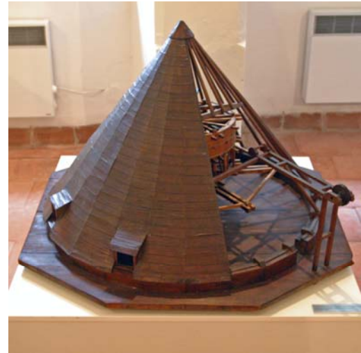
Machine for lifting ores. Diagrams from De Re Metallica and photos of model in the Mining Museum in Jachymov
